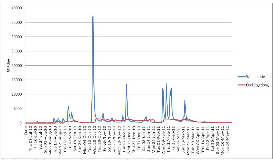
Figure 4: 2010/11 flood event - Walbundrie flow gauge compared to Cocketgegong flow gauge
