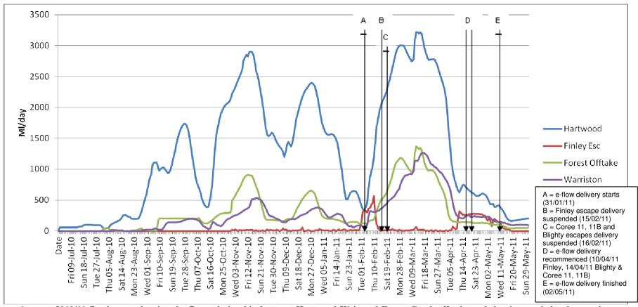
Figure 6: 2010/11 flood event showing the flow relationship between Hartwood Weir and Forest Creek off-take and the time periods when environmental water was delivered into the system
